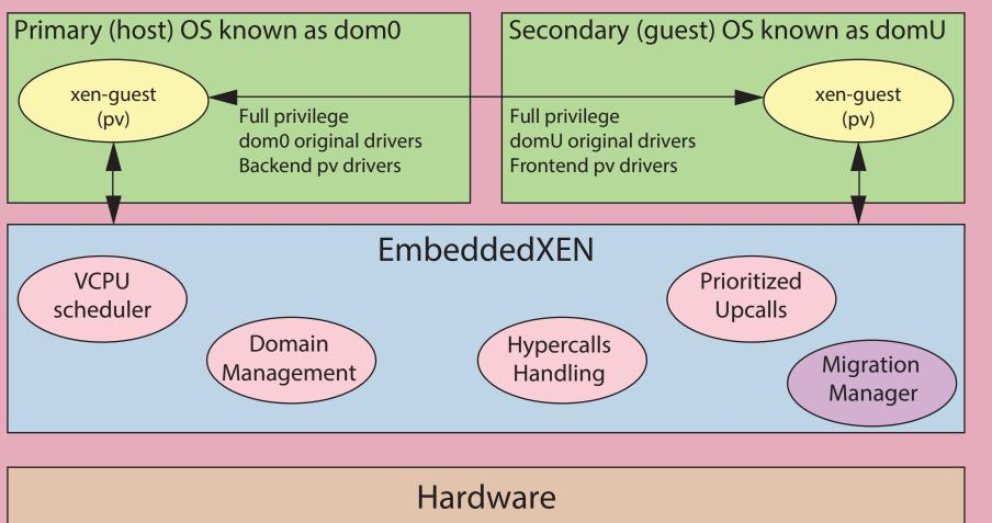
EmbeddedXen provides a virtualized hardware interface to the third-party OS. EmeddedXen supports ARM CPU cores v5-v6-v7, two (Linux-based) running OS instances, single kernel binary image easy to deploy and Virtualized interfaces for UART, block device, network, framebuffer, touchscreen and audio.
